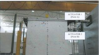
Figure 3: Two double actuator were fixed to top of wall panel
