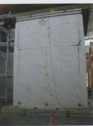
Figure 5: Cracks Patterns after testing at Wall 2
